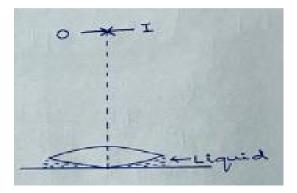
b) If r = 10 cm, a = 15 cm and b = 10 cm, find the refractive index of the liquid.
